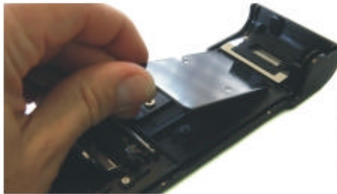
Fig. 2 start removing the pressure plate
