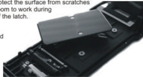
Fig. 3. Rotate pressure plate clockwise to remove.
