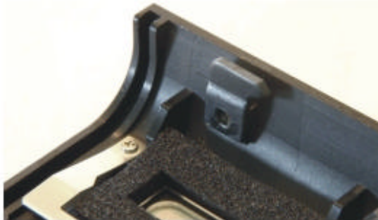
Fig. 8. New latch is glued to the base of the old latch
